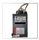
Raynor FireHoist FSEP operators offer  $\frac{1}{3}$  hp,  $\frac{1}{2}$  hp, and 2 hp planetary reduction gear drive providing an integrated fire door system. Resetting of the operator is as easy as activating the open control to reset the door with the exception of melting a fusible link. The FSEP models are also available for retro fitting existing fire doors by eliminating all the components that typically fail with an operator.
